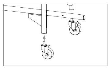
**4.** Once frame is complete, thread casters into bottom of uprights. Place locking casters on opposite sides.
