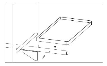
**5.** Apply large flat shelf onto extension bars. Secure to extension crossbars under shelf with hardware provided.
